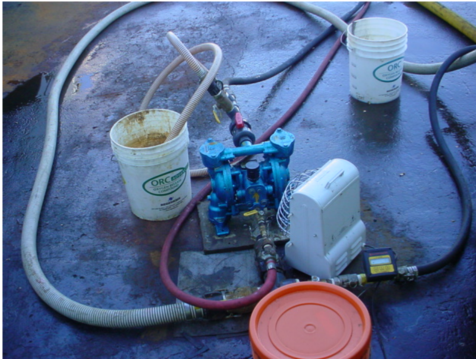
Photograph: 3 Injection pump, receives sodium persulfate solution from the mixing tanks and injects into drive rods at each injection boring.
