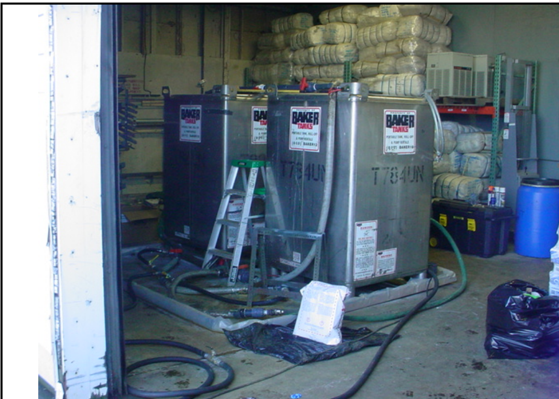
Photograph: 2 Sodium persulfate mixing tanks (tank capacity = 550 gallons each). Spokane ANG5 ERM 242 nd CCSQ Spokane, WA
