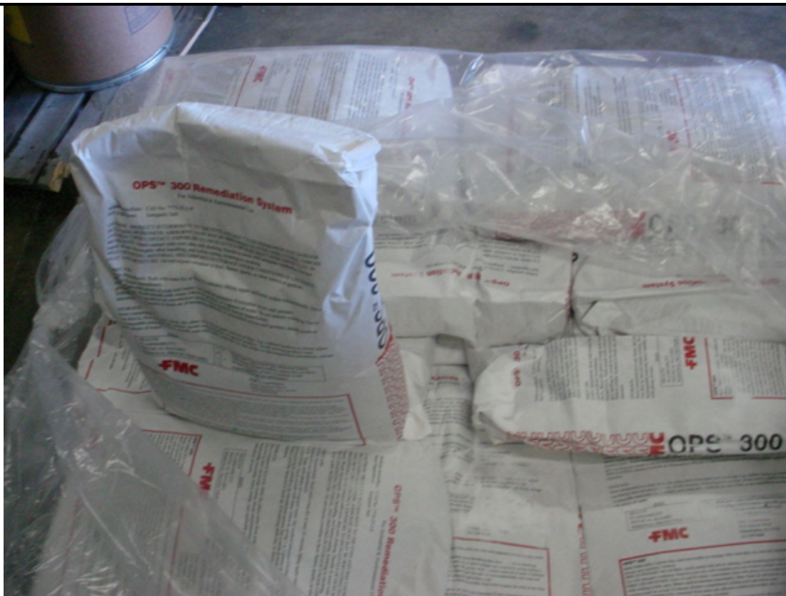
Photograph: 1 Sodium persulfate in powder form, ready for mixing. Spokane ANG5 ERM 242 nd CCSQ Spokane, WA
